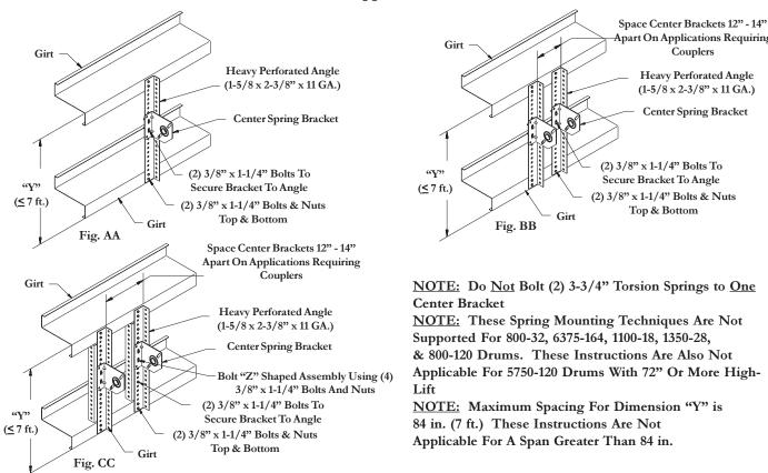
Maximum Door Size 9' x 9' (Maximum Door Weight 210 lb.) Fig AA: Cut perforated angle (1-5/8 x 2-3/8" x 11 GA.) to Dim "Y". Thru-bolt top and bottom of angle to each girt using (4) 3/8" x 1-1/4" bolts and nuts. Thru-bolt center bracket to perforated angle using (2) 3/8 x 1-1/4" bolts and nuts (See Fig. N-2).
